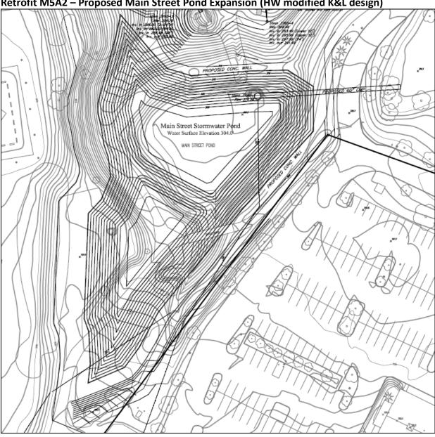
Retrofit M5A2 – Proposed Main Street Pond Expansion (HW modified K&L design)
